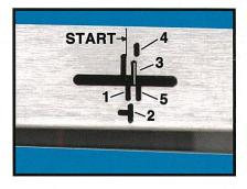
Step 7: Determine the required slot for your drive from Table 1. Tighten the belt until the line has moved to the designated slot. (In this picture the line is in Slot 3.)
