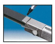
**Step 6:** Scribe a line at the spring end of the Tension-Finder. Use this line as a reference point in case the spring slips off the belt.
