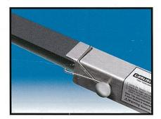
**Step 5:** With the line in the Start Slot attach the spring to the belt. Note: For cog belts the best place for the spring may be in a cog. See special instructions on page 2.
