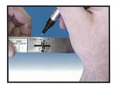
Put a dot at the Start Slot. Be careful not to catch the pen in the slot--you may pull the tip out of the pen.
